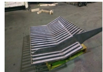
AR Steel Grate/Screening
